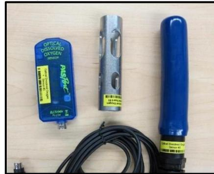
Figure 1. Dissolved oxygen handheld probe (PASCO).
