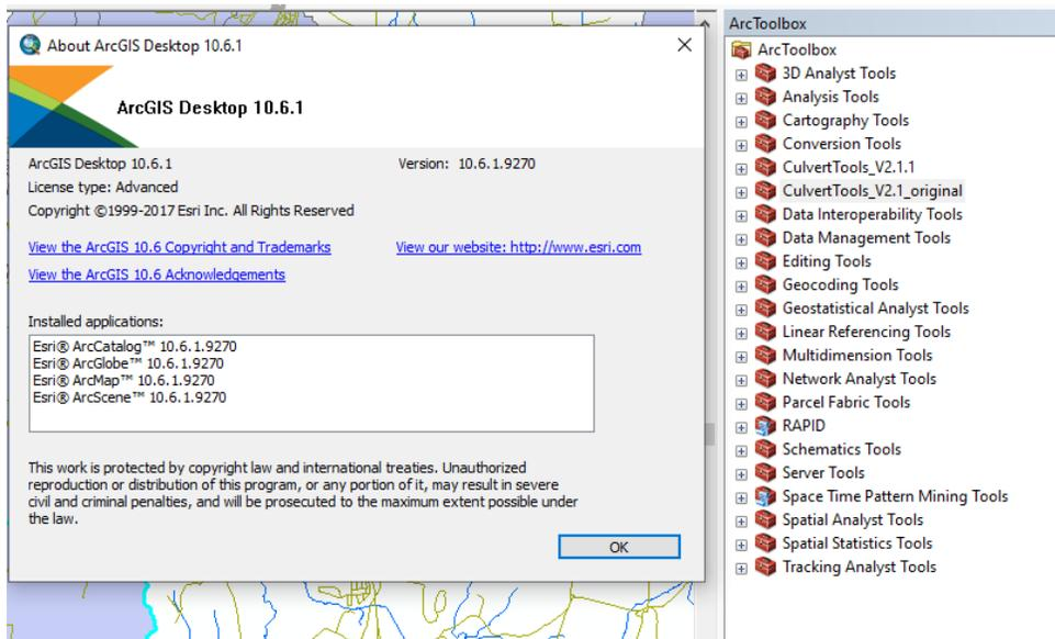
The ArcGIS Toolbox “CulvertTools\_V2.1”, had several errors of unknown origin when installing using ArcMap 10.6.1. Several of the ArcMap models within the toolbox were modified slightly in ArcMap 10.6.1 and the result saved as “CulvertTools\_V2.1.1”.
