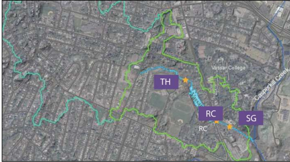
Figure 2 The urbanized headwaters of the Fonteynkill, with the above-ground watershed (light green), the presumed urban storm drainage (blue-green), and the three sonde sites.
