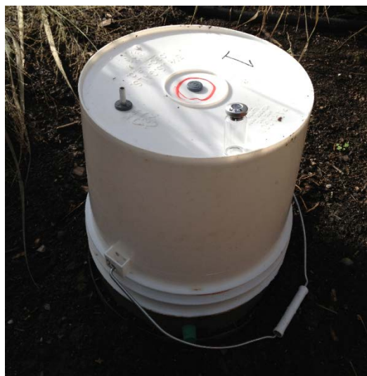
Figure 2. Photograph of static chamber configuration
