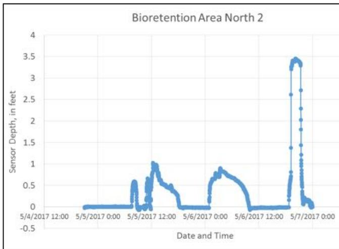
*Figure 3: Example of a hydrograph from Bioretention Area North 2, which does not have an underdrain, between May 5 and May 7. Values are recorded every minute, and converted from pressure to sensor depth by HOBOWare software based on barometric pressure.*
