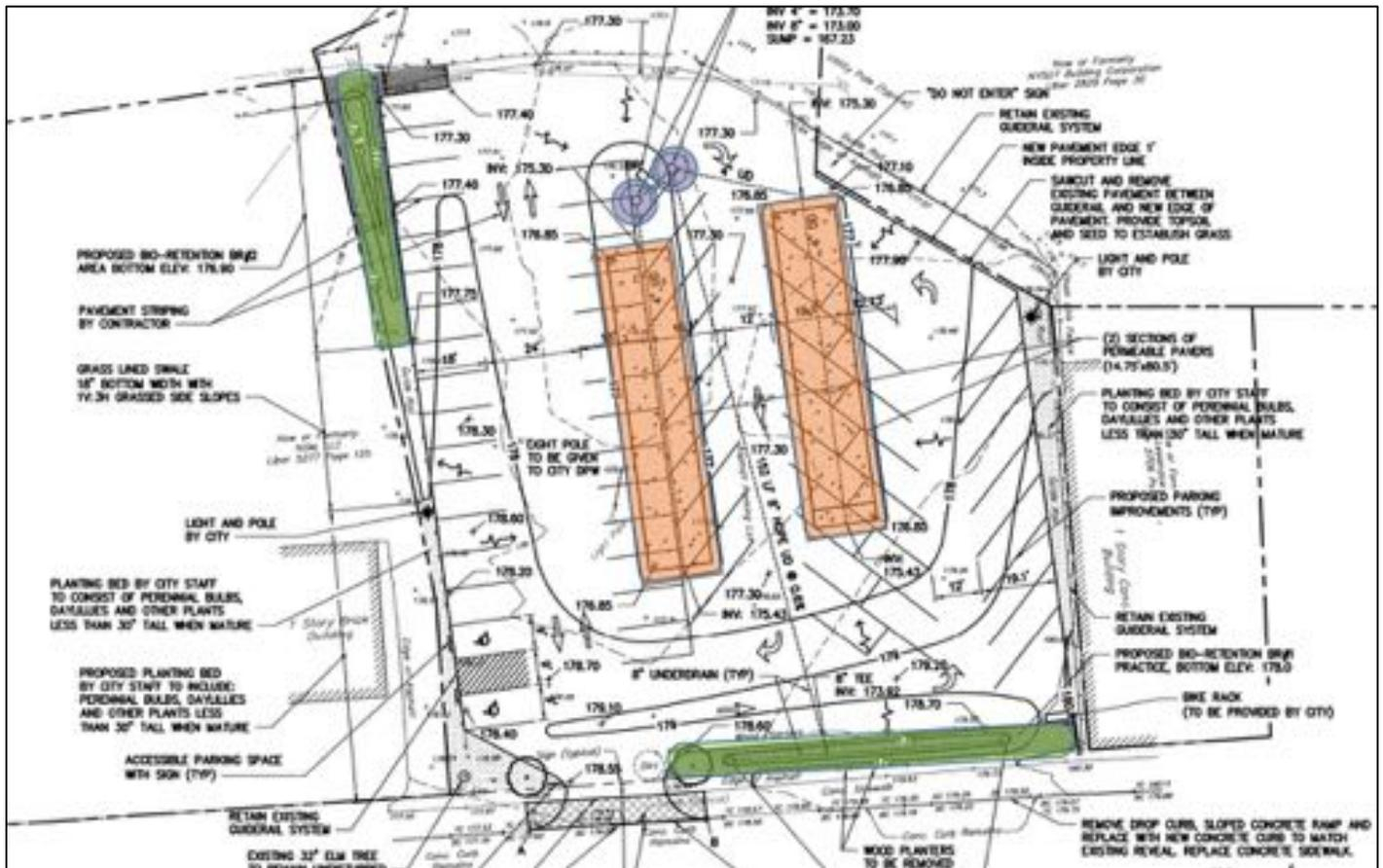
Figure 2: Engineering plans for the North lot, with bioretention areas (green), pervious pavers (orange), and dry wells (purple) highlighted (Barton & Loguidice 2015).
